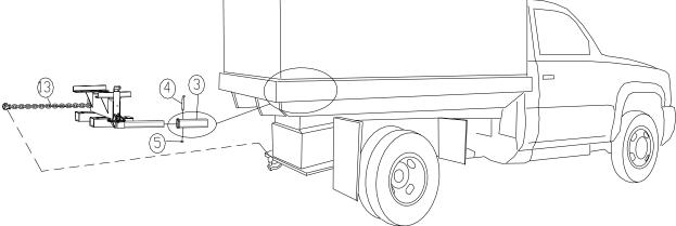
Item 3, tube truck, is to be installed by welding it to the side frame of the truck. Exact position will be determined by the individual user's collection box position.
