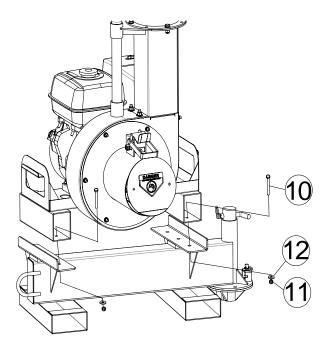
Attach the DL to the hitch using the hardware provided.
